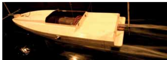
Fig. 8. High-speed navigation at 13 m/s without air jets
