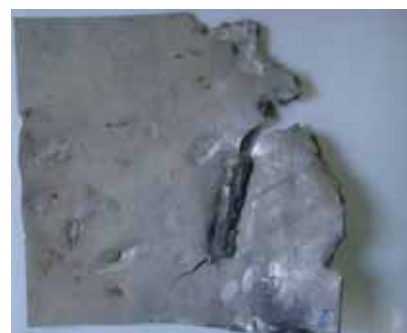
Fig.9. Effects of 7020M alloy sheet perforation (dimensions 300x3000): a) homogeneous g = 12 mm b) split (w-inner, z –outer from the source of explosion, total thickness g = 2x6 mm) after detonation of high explosive shell of OF412 type and calibre 100 mm with the contents of 1,4 kg of TNT, taking place at a distance of 0,6 m.
