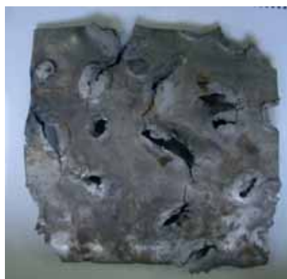
Fig.9. Effects of 7020M alloy sheet perforation (dimensions 300x3000): a) homogeneous g = 12 mm b) split (w-inner, z –outer from the source of explosion, total thickness g = 2x6 mm) after detonation of high explosive shell of OF412 type and calibre 100 mm with the contents of 1,4 kg of TNT, taking place at a distance of 0,6 m.
