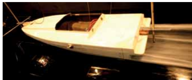
Fig. 7. High-speed navigation at 13 m/s with air jets
