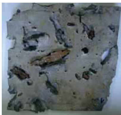
Fig.9. Effects of 7020M alloy sheet perforation (dimensions 300x3000): a) homogeneous g = 12 mm b) split (w-inner, z –outer from the source of explosion, total thickness g = 2x6 mm) after detonation of high explosive shell of OF412 type and calibre 100 mm with the contents of 1,4 kg of TNT, taking place at a distance of 0,6 m.
