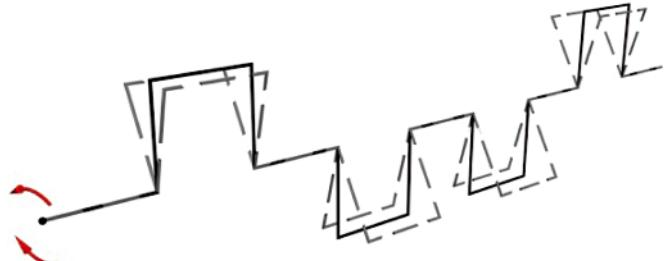
Fig. 9. Torsional crankshaft vibration
