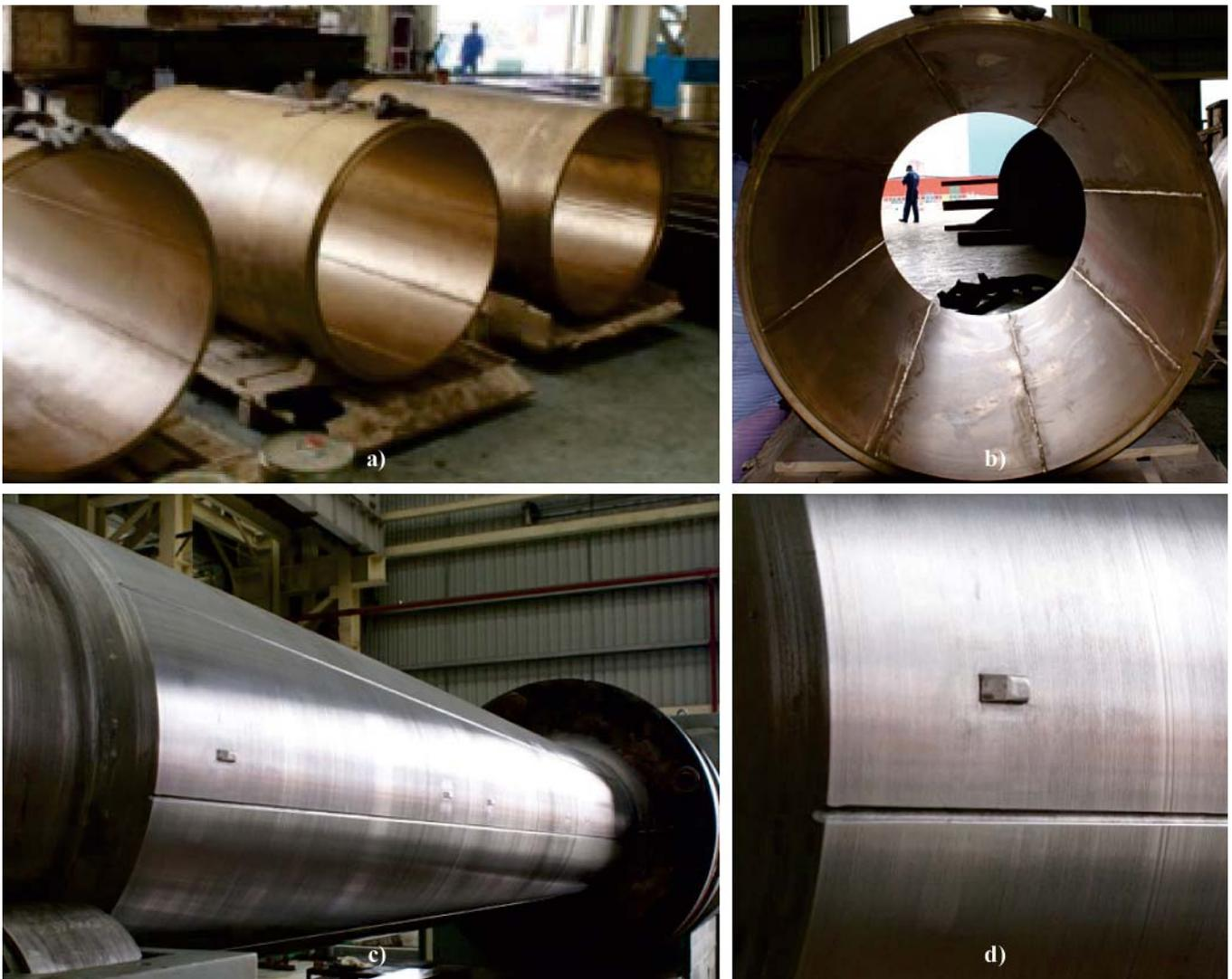
*Fig. 5. Sections of the bearing sleeve and the shaft with cut splineways and welded spacing elements*
